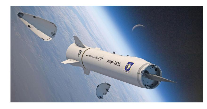
The Tactical Boost Glide (TBG) vehicle developed by the Defense Advanced Research Projects Agency forms the basis for the hypersonic boost-glide missile that the Air Force is developing, the Air-Launched Rapid Response Weapon. The TBG is shown here as a slender, pointed object on the front end of the missile. The cone in the upper left of the drawing is the protective shroud from the front of the missile, which has just been ejected in preparation for releasing the TBG.
