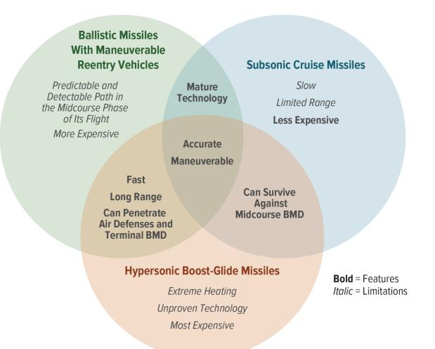
The hypersonic missiles being developed by the U.S. military combine desirable traits of two types of U.S. missiles with welldeveloped technology: ballistic missiles' speed and long ranges, and subsonic cruise missiles' maneuverability and ability to survive against midcourse missile defenses. Hypersonic missiles introduce new technical challenges, however.
