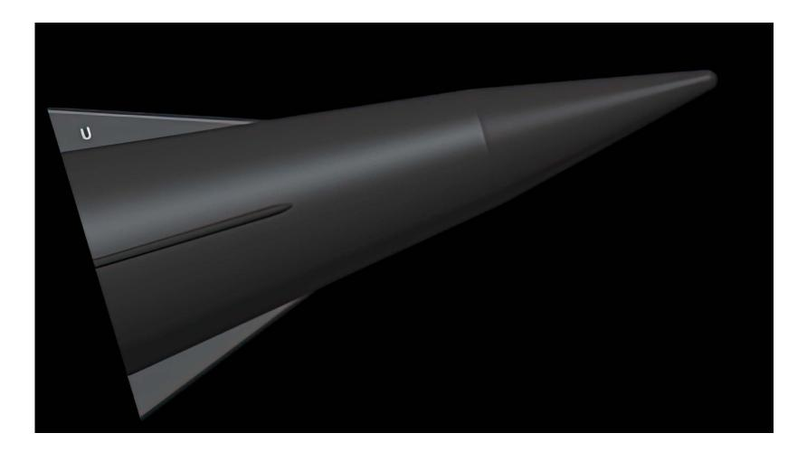
The Army and Navy are collaborating on the Common Hypersonic Glide Body (C-HGB), the part of a hypersonic boost-glide missile that detaches from the spent rocket booster and glides to its target. Both services plan to use the C-HGB in the hypersonic boost-glide missiles they are developing: the Army's Long-Range Hypersonic Weapon and the Navy's Intermediate-Range **Conventional Prompt Strike** missile.
