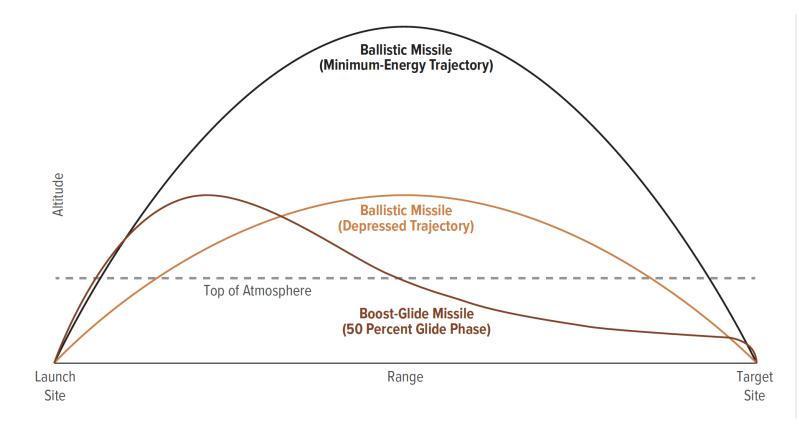
A missile's ballistic trajectory can be shaped in many ways. This figure shows a simple minimum-energy trajectory that is very close to a parabola, influenced mainly by gravity after the missile's rocket booster burns out, and a depressed trajectory, when the ballistic missile is launched at a shallower angle.
