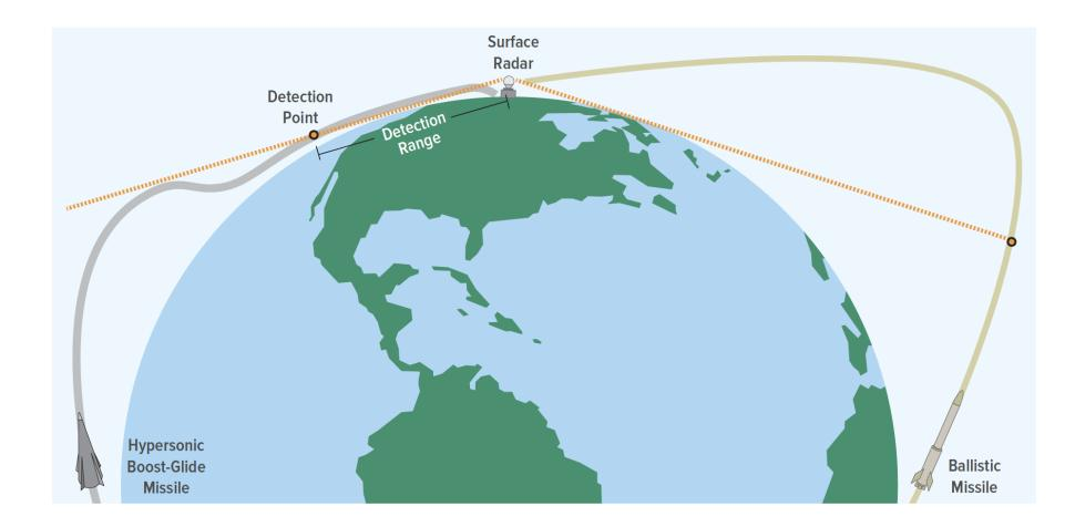
Because of the curvature of the Earth, a radar cannot detect a missile that is below the horizon. The distance to a radar's horizon increases with the height of the radar's antenna and the altitude of its target.
